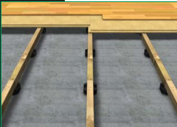
Typical floor system configuration..
