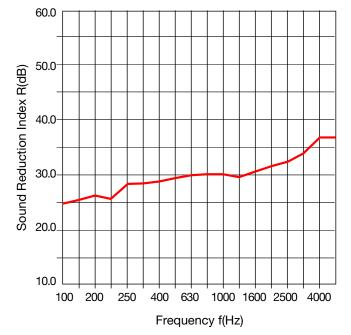
Test results for JCW Reflective Sound Screen issued by: University of Salford (Acoustics Test Laboratory) UKAS accredited test laboratory No. 1262
