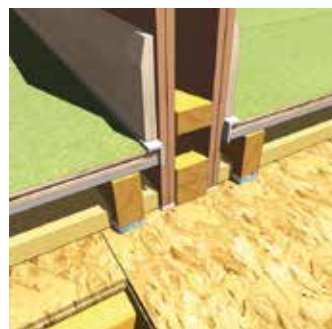
Internal Wall Junction (Loadbearing)
