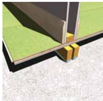
Support of Non-Load Bearing Partitions
