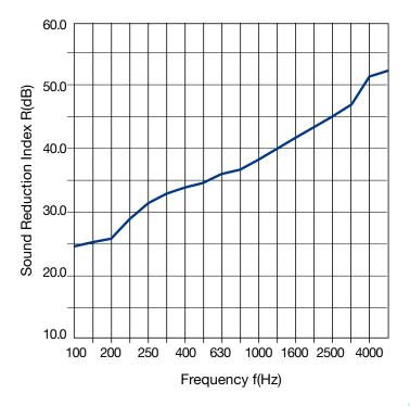
Test results for JCW Absorbent Sound Screen issued by: **University of Salford (Acoustics Test Laboratory)**UKAS accredited test laboratory No. 1262
